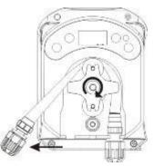
Step 2- Turn the roller clockwise and release the (left) intake ring nut
