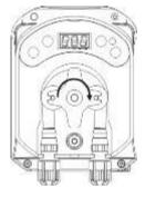
Step 4 - Release t the (right) delivery ring nut and remove it completely
