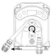
Step 2- Turn the roller clockwise and release the (left) intake ring nut
