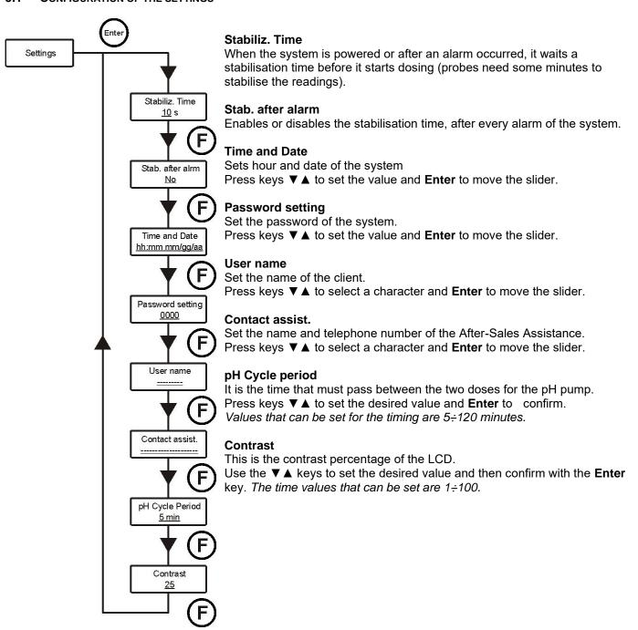
To confirm and exit, press key Enter for 3 seconds.
