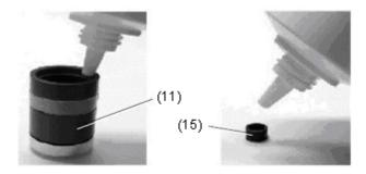
Fill (11) and (15 only for ADELCLJ15) with the electrolyte supplied, making sure not to create air bubbles.
