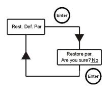
The restoration of the factory parameters is enabled (refer to appendix 1). The system asks if you are sure to proceed.
