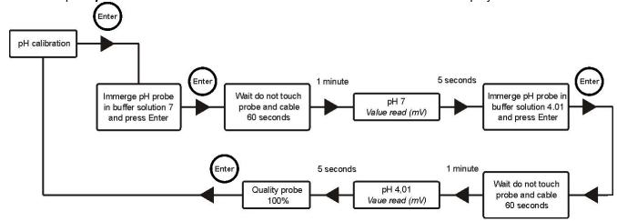
Once carried out the pH 7 calibration, rinse the electrode with water, so to prevent the pH 4 solution from polluting.
