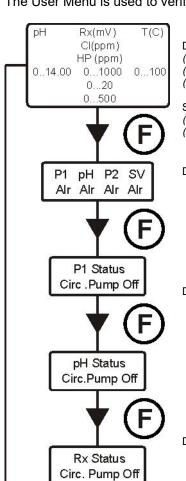
EV Status Circ. Pump Off Default screen shows the reading of the pH and Rx or Cl or HP and the temperature. (redox in mV is displayed on Time/pH/Rx and pH/RxTechnopool3). (the chlorine in ppm is only displayed on the Technopool3 pH/ClJ). (the hydrogen peroxide in ppm is only displayed on the Technopool3 pH/HP).
