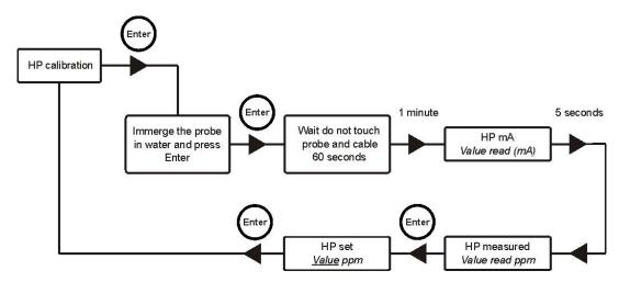
When the system acquires the calibration value, two parameters regarding the measure are displayed:
