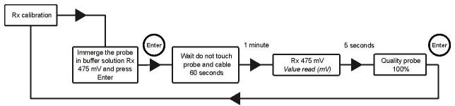
Once the procedure is completed, the quality of the calibrated electrode will be displayed; if the quality of the probe results 25% or less, carry out a new calibration.
