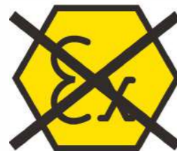
No explosion proof equipment
