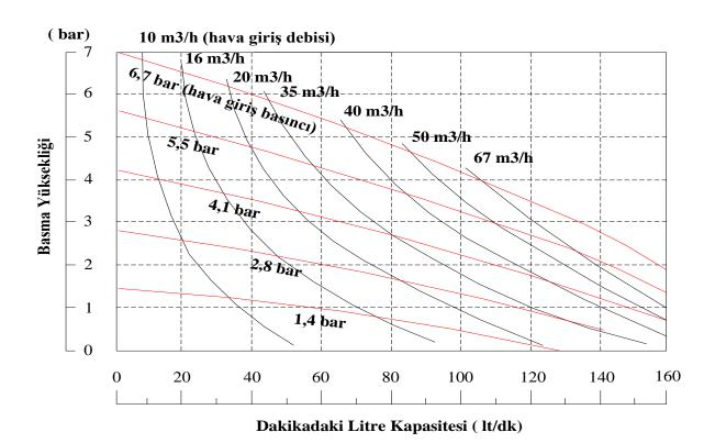
Suction / Discharge 1" Max. Capacity 160 lpm Max. Solid particle (4 mm) Max. Operation pressure 8,4 bar Weight 9 kg (AL)
